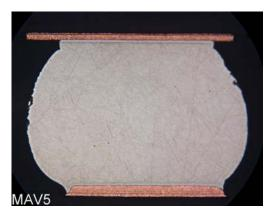
Figure 19 - Maverick Card #5 Double Rework on the Maverick Card OSP, 304 Pin BGA at U29.
